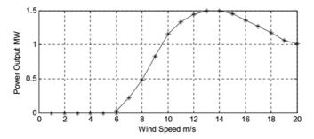
Fig. 3. Power curve for model
